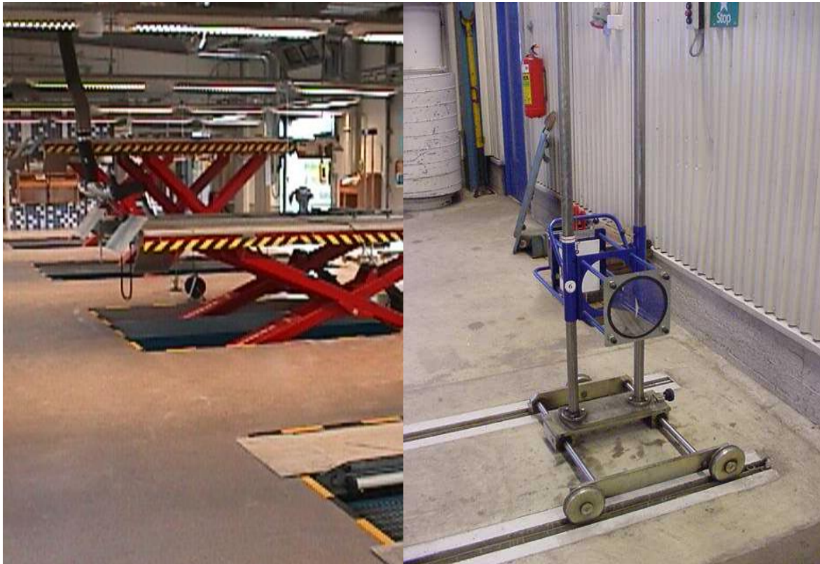
Typical lift and equipment for testing lights:
