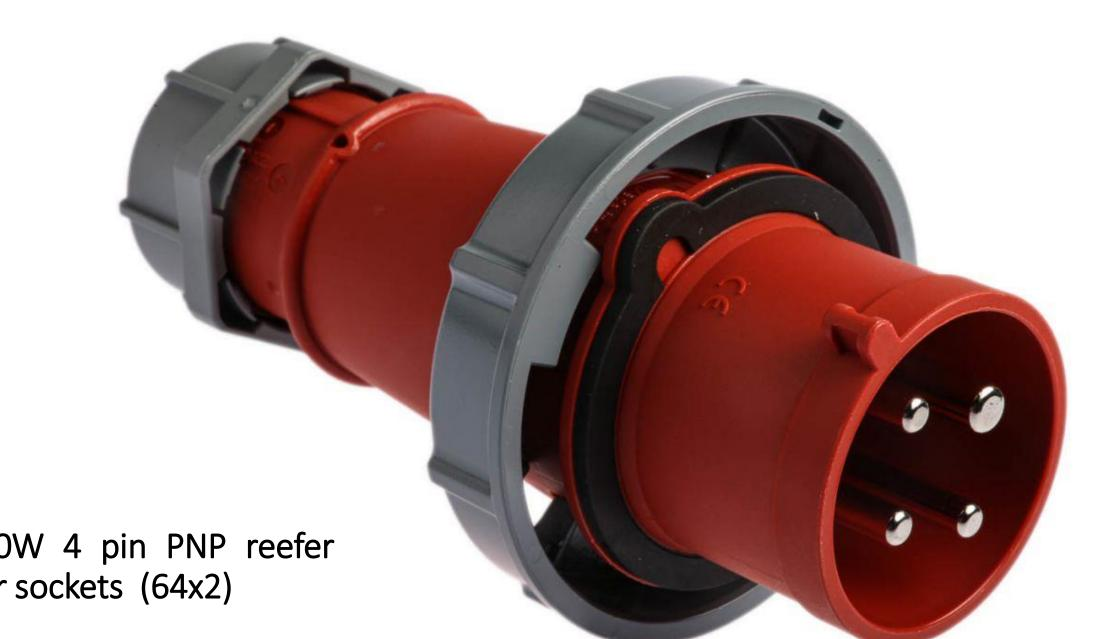
Supply and install 32A, 4 pin, 380-440 acV and 50-60 Hz reefer power outlet as MENNEKES IP67 (type 5946A) with running hour meter as AC/DC DYNAMICS(SQ48R) or equally approved
